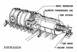
CUTAWAY DRAWING of HERMES II shows internal components. Circular hatches on sides and top of tank are for access. Small windows are located at center of these.
